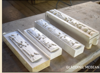
Left: Initial test run output showing the evolution and refinement of our use of CNC. The model on the far right proved that this process could provide ornate modeling that is production ready. Right: Examples of Plaster models created using CNC and used for production.
