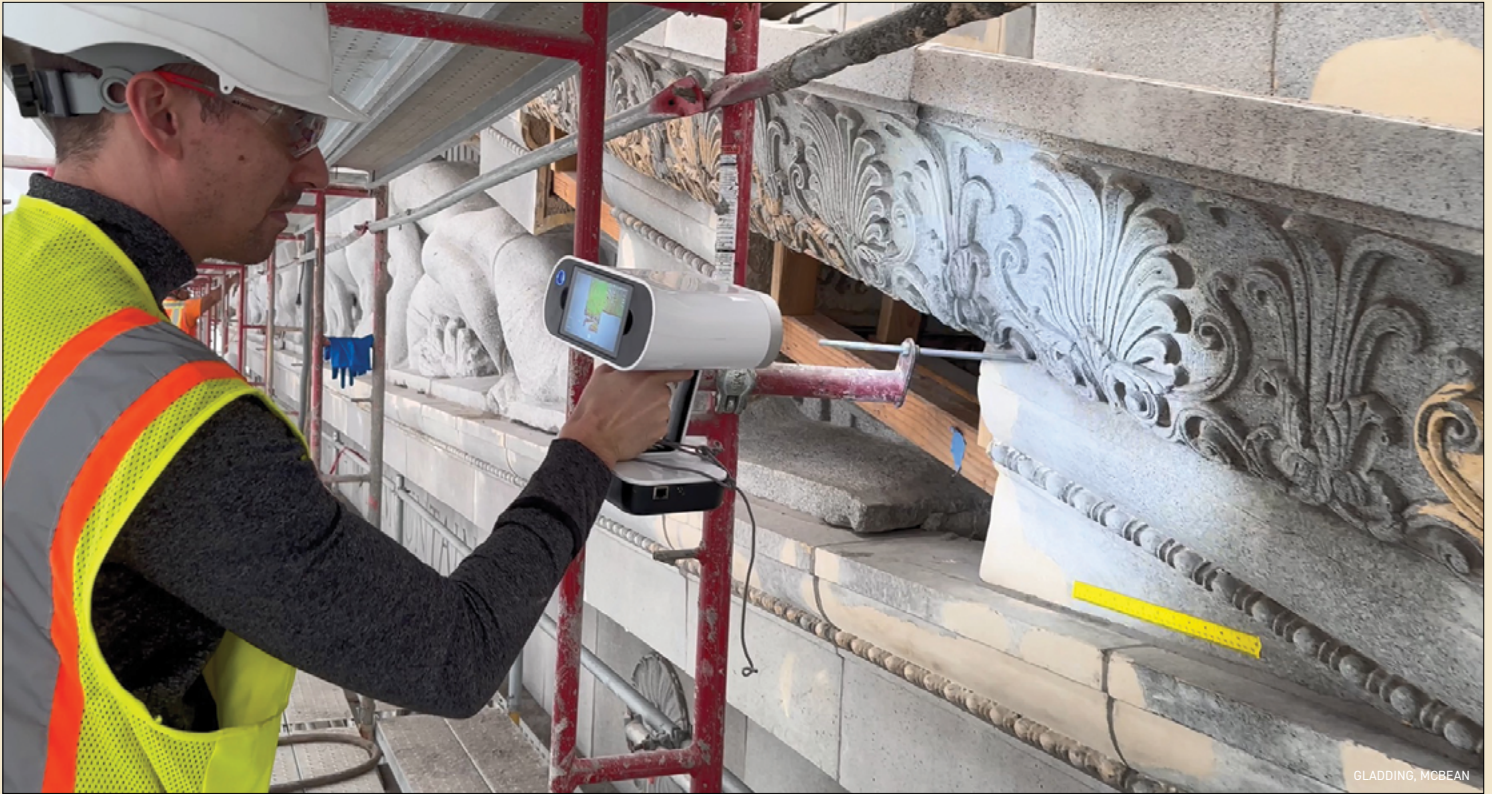
Above: A member of the Gladding, McBean Drafting and Survey Team operating a handheld scanner at a jobsite. Below: The 3D model created directly from the scans gathered in the field.
