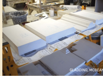
Left: Initial test run output showing the evolution and refinement of our use of CNC. The model on the far right proved that this process could provide ornate modeling that is production ready. Right: Examples of Plaster models created using CNC and used for production.
